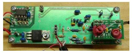
This is one of the Softrock RX kits built up as a single band unit. There is a switched Bandpass filter unit available, which allows reception across 1.8 thru 30 MHz. A new Programmable Oscillator IC allows tuning of the RX across
